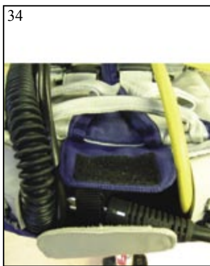
34- Ensure that the power inflator/hose is on the opposite side of the opening to the other hoses
