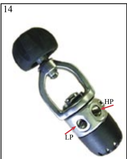
14- Remove the L/P port plug to the left of the H/P port as shown. Use this L/P port plug to seal the port from where the L/P hose/second stage was removed
