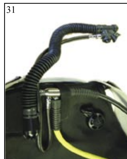
31- Attach the L/P inflator hose to the power inflator by pulling the sprung loaded fitting down, and inserting on top of the metal nipple which protrudes.
