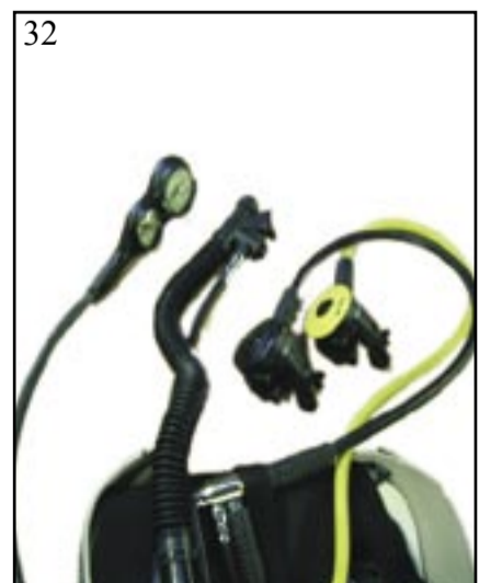
32- Pull the regulator and alternate source hoses through the top of the rucksack to the right
