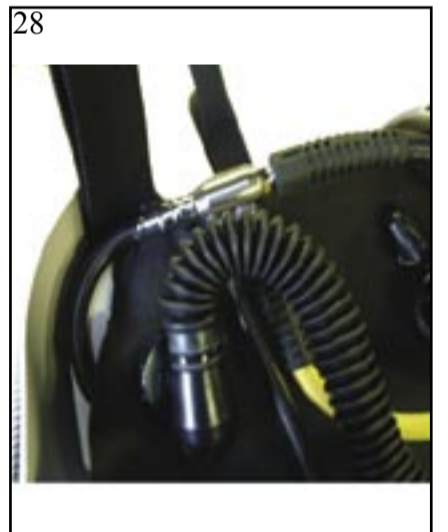
28- Position the manifold assembly at the top left hand corner of the rucksack
