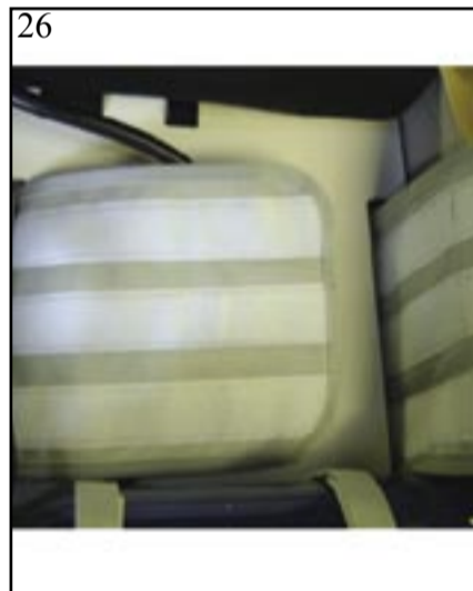
26- Separate the two halves of the weight pouch belt and place the L/P feeder hose against the support board
