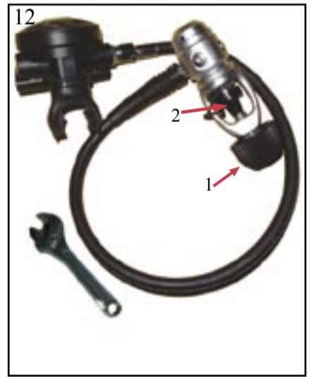
12- Unscrew the yoke *1* and remove the dust cap *2*. Remove the L/P hose/second stage from the regulator first stage
