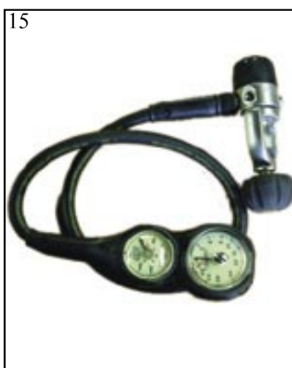
15- Screw the H/P hose of the depth/pressure gauge into the high pressure port
