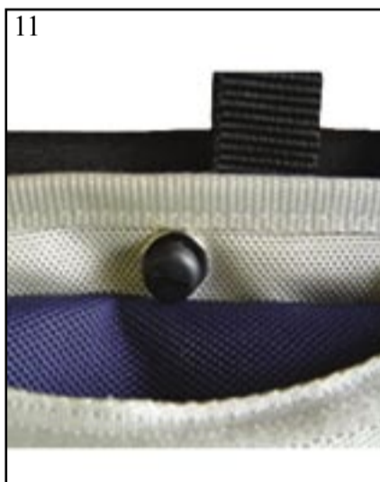
11- Push the securing bolt through the metal eyelets of the rucksack and the air cell into the nut embedded in the support board and tighten
