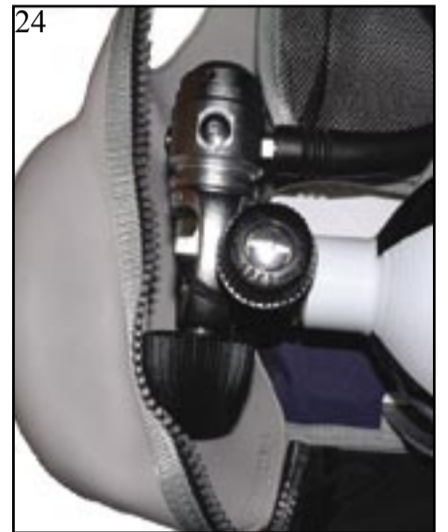
24- Attach the regulator first stage to the cylinder valve with the L/P feeder hose pointing downwards, towards the support board
