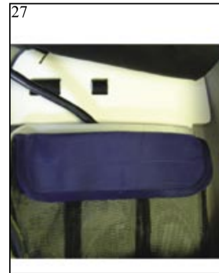
27- Fold the two halves of the weight pouch belt together on top of the L/P feeder hose. which must point towards the top left hand corner of the rucksack
