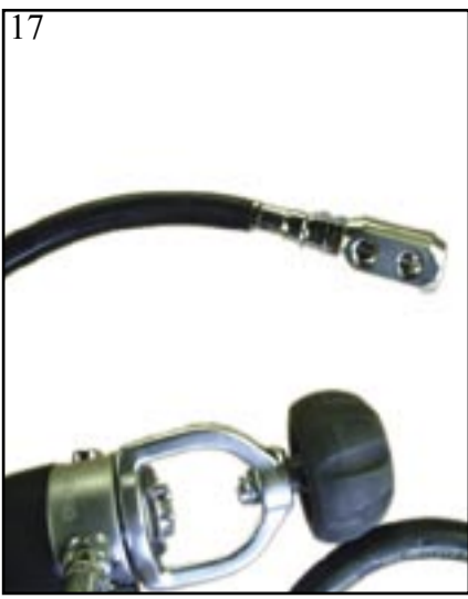
17- Attach the male threaded end of the manifold to the feeder hose
