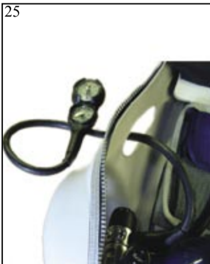
25- Push the depth/pressure gauge hose through the slot in the left hand side of the rucksack
