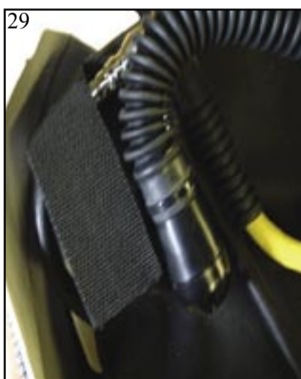
29- Secure the L/P feeder hose in place with the wide hose retaining strap
